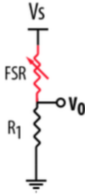
Figure 2.2: Voltage Divider conditioning circuit used for FSR [1]
