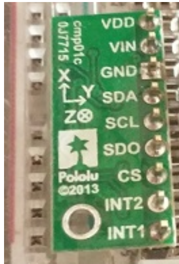
Figure 2.1: Image of accelerometer used in The Batons
